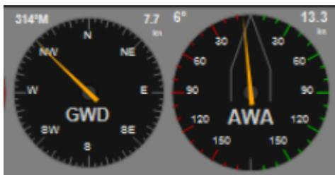
All the Wind Panels require an NMEA 0183 or NMEA 2000 compatible wind vane and anemometer to be connected to the PC and some require your speed over ground, course over ground, and heading information as well.
